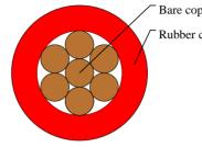
Bare copper conductor Rubber compound insulation
